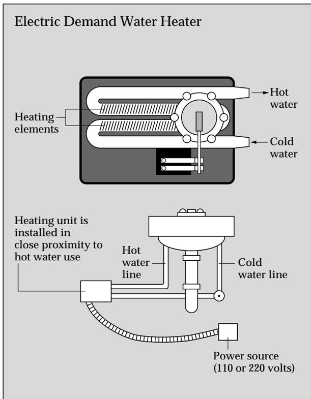
Because demand water heaters have no storage tanks, standby heat losses are completely eliminated.
